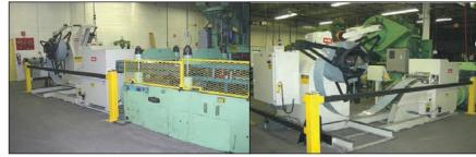
forced straight up into the guide chute on the entry end of the straightener/feeder for hands-free threadup. The straightener/feeder unit is also supplied with pneumatic roll release to allow the upper feed and
