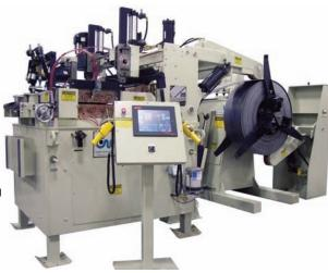
Right: 609 mm x 6.35 mm x 4,530 kgs Compact Coil System with touch screen interface
