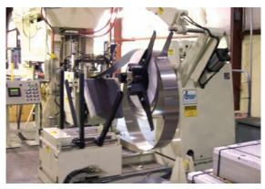
straightening rolls to open and allow the pilots to register the material into position.
