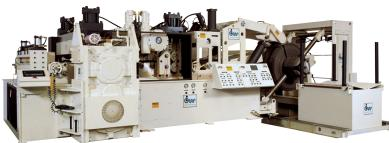
The press feed system has the capacity to handle materials from 1.22mm through to 6.35 mm thickness up to 1524mm wide, with the ability to process 12.7mm thick material up to a width of 762mm. A key consideration was the wide variety of coils with yield strengths ranging from a low of 413n/m<sup>2</sup> to a high of 827n/m<sup>2</sup>, which the system would have to process.
