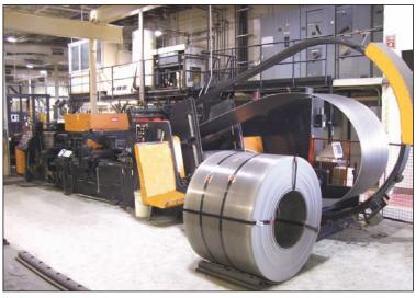
For short run, partial coil operations, Formtek has designed a compact system to handle 609 mm x 6.35 mm x 4,535.90kgs. The CWP system features a motorized uncoiler with photo eye loop control to allow the slack material to develop directly below the uncoiler spindle. Both primary and secondary hold-down arms are provided with powered rider rolls for thread-up and to allow for rewinding the slack material during partial coil operation.
